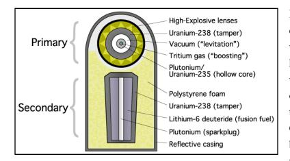
Fission weapons are sometimes called atomic bombs, while fusion weapons are also known as hydrogen bombs or thermonuclear weapons. The basic components of a fusion weapon are shown in this diagram (source: Wikimedia Commons). The "primary" is basically an implosion fission weapon that is used to ignite the
