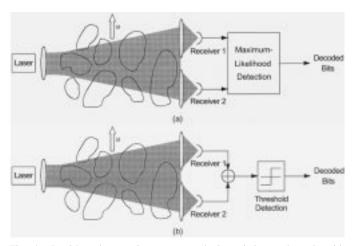
Fig. 4. Dual-branch reception on atmospheric turbulence channels with correlated turbulence-induced fading. (a) Maximum-likelihood detection. (b) Equal-gain combining with threshold detection.
