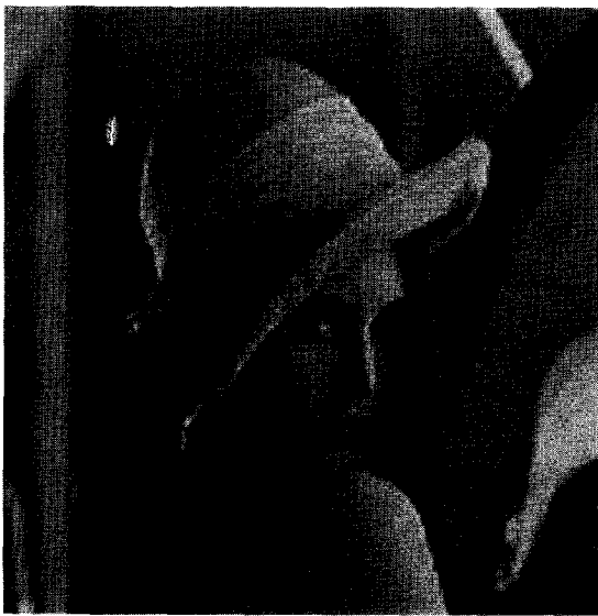
Fig. 8. Subband coded image of rate 0.25 bpp. The PSNR of the image is 29.24 dB.
