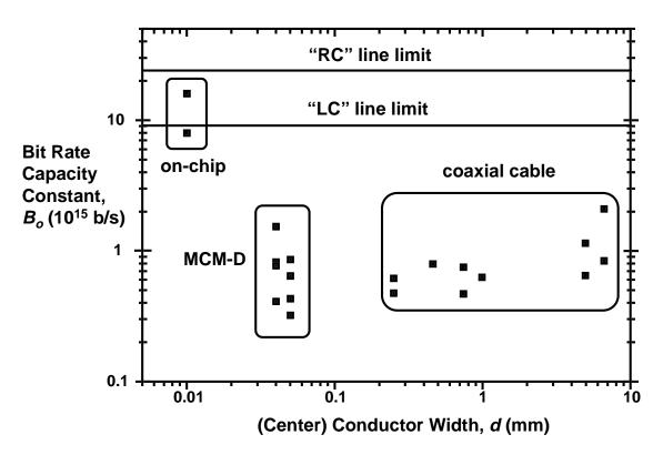
Fig. 4. Bit-rate capacity constant for various cables and transmission lines, as a function of the cross-sectional dimension, *d*, of the smaller conductor in the line.
